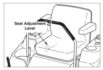
Figure 28. Seat Adjustment
